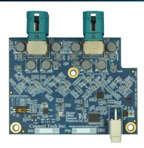
Since many different types of GMSL cameras are available, the JCB002 has user selectable options to interface with either GMSL1 or GMSL2 protocols at different operating frequencies.
